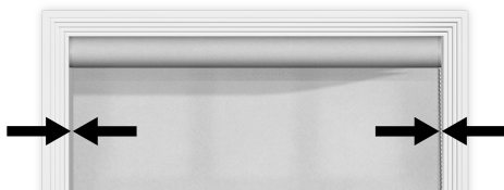
Inside Mount Light Gap (Refer to light gap chart.)
